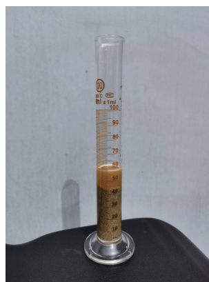
图3 遇水固结型支撑剂在煤油中24 h溶解 Fig. 3 Consolidated proppant dissolved in kerosene after 24 hours
